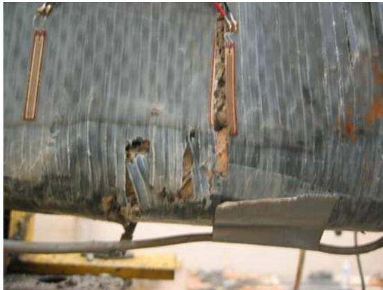
a) CFRP sheets rupture
