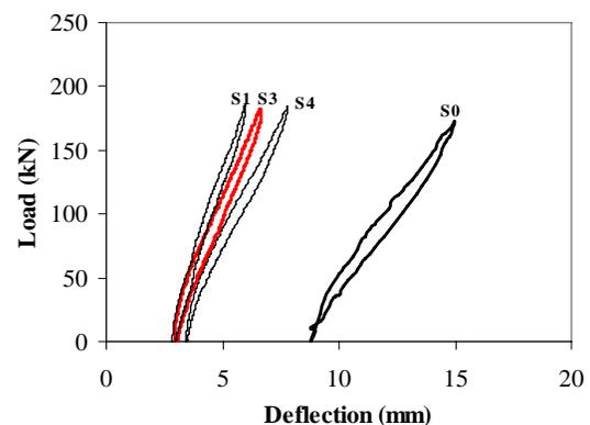
Fig. 3: Comparison between static responses of test prototypes after different fatigue loading steps
