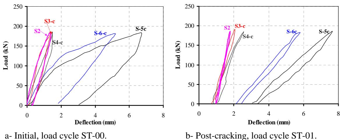
Fig. 4: Initial and post cracking load-deflection responses of test prototypes
