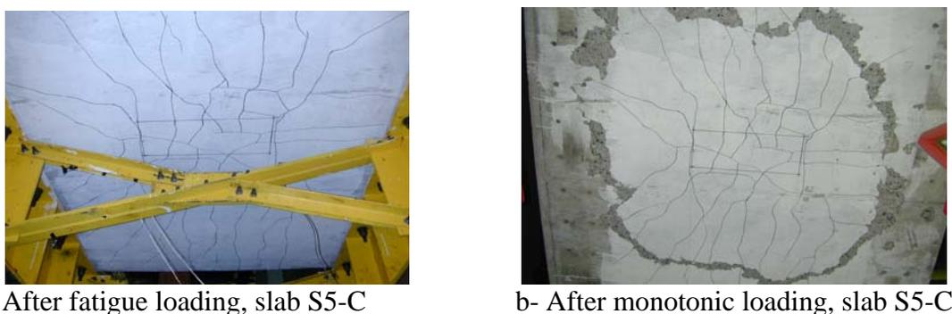
Fig. 7: Comparison of crack patterns on the bottom surface after different loading
