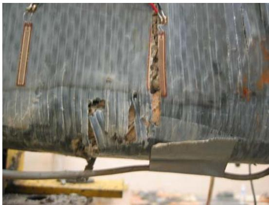
a) CFRP sheets rupture
