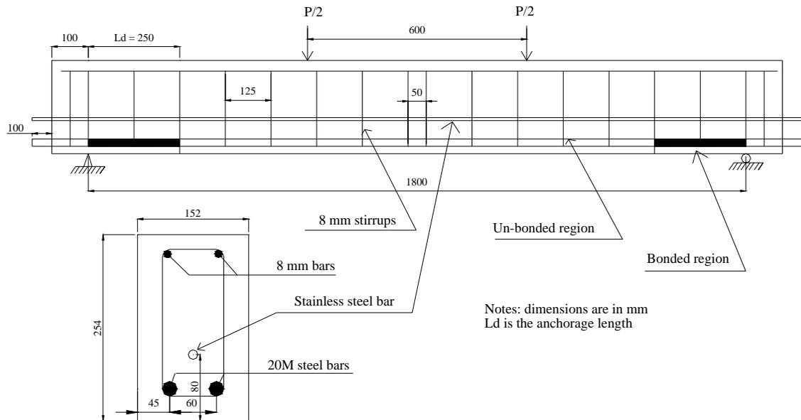
Fig. 1: Longitudinal and cross sectional details for the bond-beam specimen.
