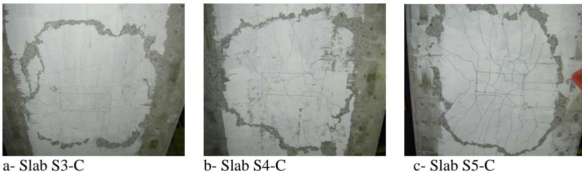
Fig. 6: Comparison of failure shapes and crack patterns on the bottom surface.
