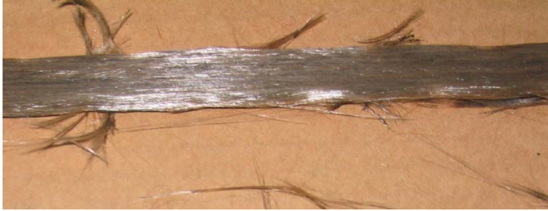
Fig 17 The middle of a G2 rod after resin burn-off showing revealing straight glass fibres.
