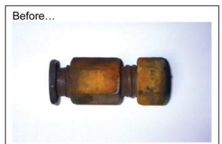
Dip your steel parts into any container with RustRelease™ and let the solution do its work. This usually takes 15 minutes for light rust, and a few hours for heavily rusted steel.
